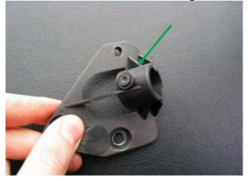
We take off black delta and unscrew the last keeping mirror screw. We draw out from thin lines of regulator the rubber washer.
