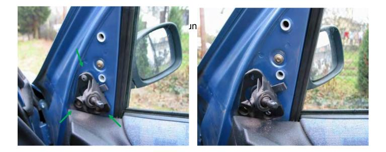
We unscrew the levers of regulator of mirror which it holds on on screw .:
